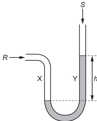
Side X is connected to a gas supply of pressure  $R$ .
